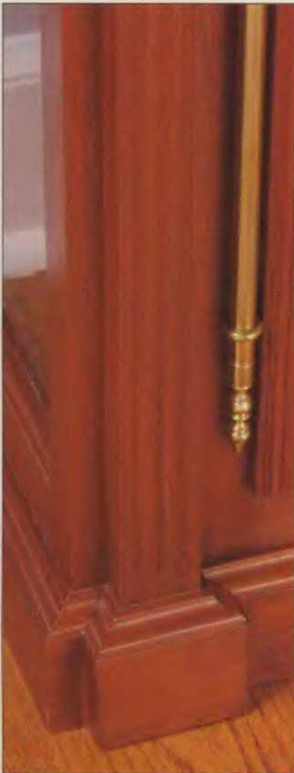
Pilasters are narrow boards fastened to the front stiles of an armoire and fluted with two or three blind grooves for decoration.
