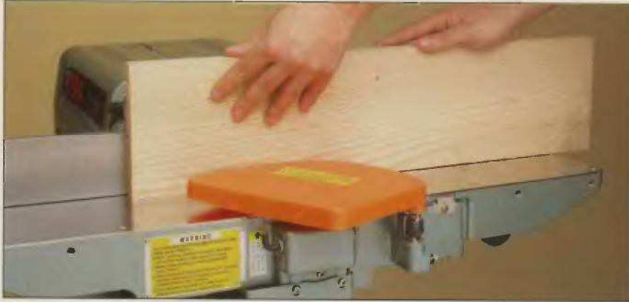
A jointer produces a smooth, even edge on a hardwood board. For best results, set a cutting depth between \frac{1}{16} and \frac{1}{8} inch.
