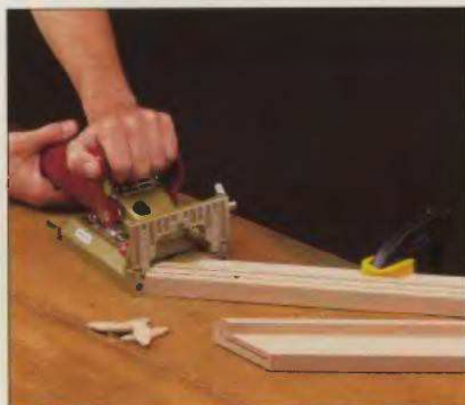
A biscuit joiner cuts a slot in the mitered end of the blanket chest's molded base. The base is rabbeted to accept the carcass of the chest and the bracket feet are then screwed to the base.
