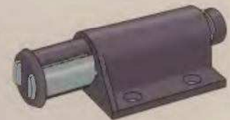
Magnetic door latch-and-plate Used with acrylic or glass doors up to 3/16 inch thick. Latch plate attaches to door and magnetic latch is mounted inside bookcase; latch holds plate magnetically, keeping door closed.
